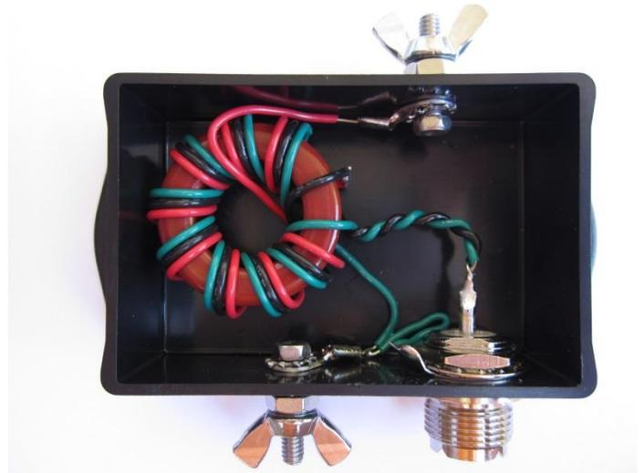
A small spot of clear silicone compound is used to secure the toroid from movement in the enclosure. The only remaining assembly step is to securely glue the box cover in place with PVC cement.
