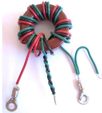
From inside the box, place an 8-32 machine screw through a lock washer, the # 8 lug on the green wire, then through the lower 11/64" mounting hole. Place a flat washer on the outside protruding machine screw followed by # 8 lock washer/nut and tighten securely. Place a # 8 wing nut on the machine screw to finish the **counterpoise connector**.
