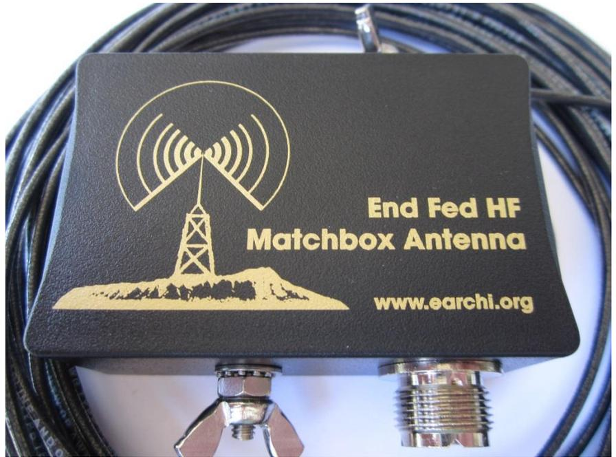
Best performance is achieved with a coax of 16' or longer with the coax shield providing the counterpoise function. Additional counterpoise is usually not required in this design, although the lower wing nut provides a convenient counterpoise connector if needed. The end fed antenna system works well in horizontal, sloper, and vertical configurations.
