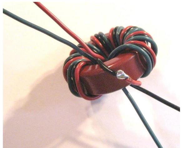
Twist the **left green** wire with the **right black** wire. Strip the ends of the two wires and twist together at about 2". This twisted pair will solder to the center connection of the SO-239 connector in a later step.
