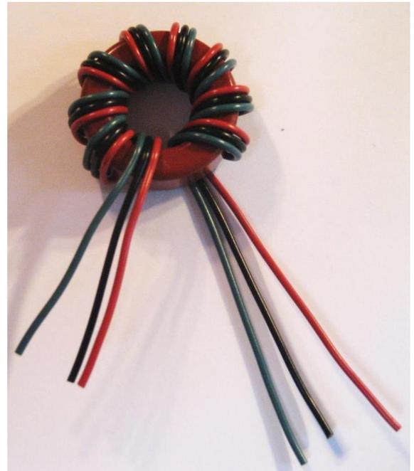
NOTE: Count turns by counting the number of times the wire goes thru the toroid center.
